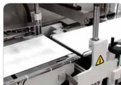
Sealing heading designed to avoid dirt accumulation
