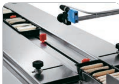
Photo cell control for "no-product no-bag" function
